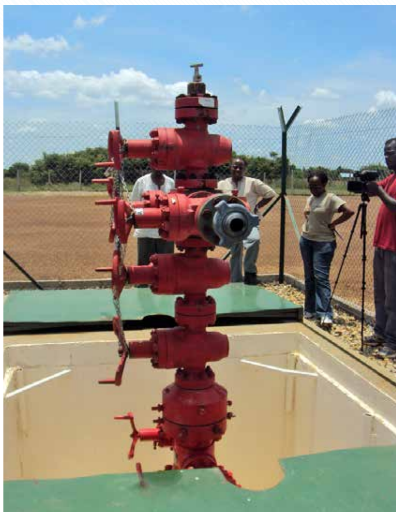
Kasemene 1 well head, one of the oil fields at field development stage
