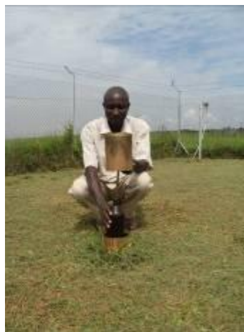
Use of manual rain gauge in Jinja – collecting drops of rain in a bottle – as the automated one is broken
