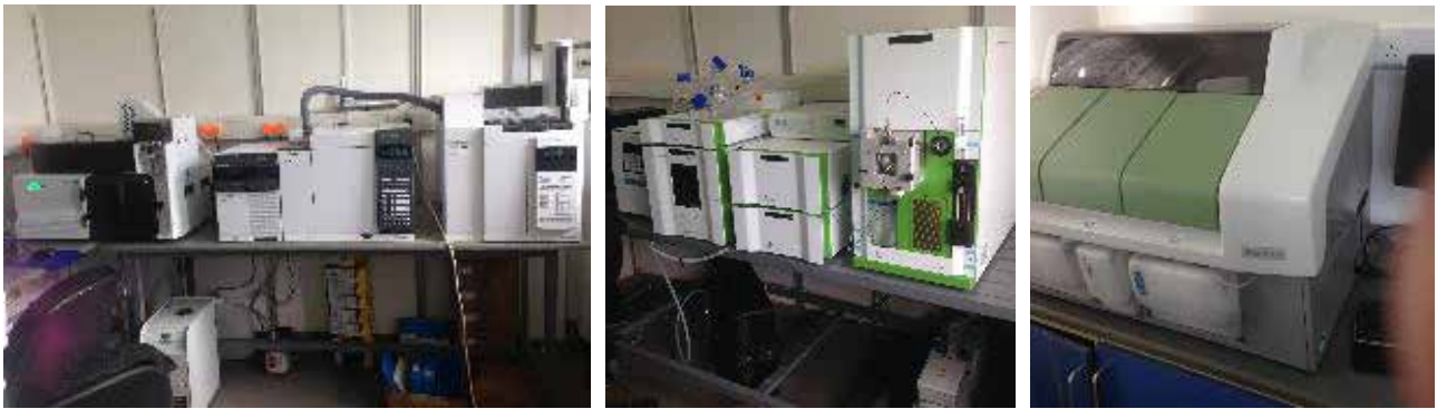
L-R: High performance liquid chromatography; Liquid Chromatography Mass Spectrometer; Gallery plus Spectrometer in Entebbe laboratory, Wakiso District
