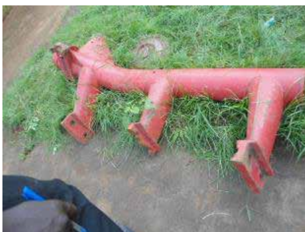
Left: Broken part of the tractor plough replaced with an old used part (R) by members of Kweyo cooperative in Omoro District
