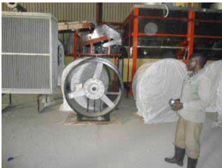
L-R: Withering fan missing blades and a transformer installed at Kigezi Highland Tea Factory in Kisoro District
