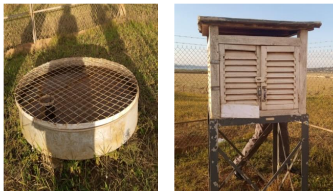
L-R: Old Evaporation Pan and a Stevenson Screen at Buku Weather Station in Entebbe
