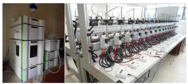
L-R: HPLC equipment at UNBS Gulu regional office and testing bench for testing energy meters at UNBS headquarters
