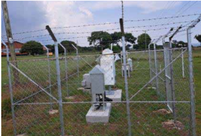
Atmospheric deposition equipment for monitoring air quality and rainfall in Entebbe
