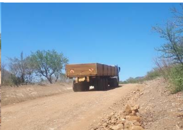
A heavy truck loaded with marble on Moroto-Lokitanyala Road. This accelerates the deterioration of the road
