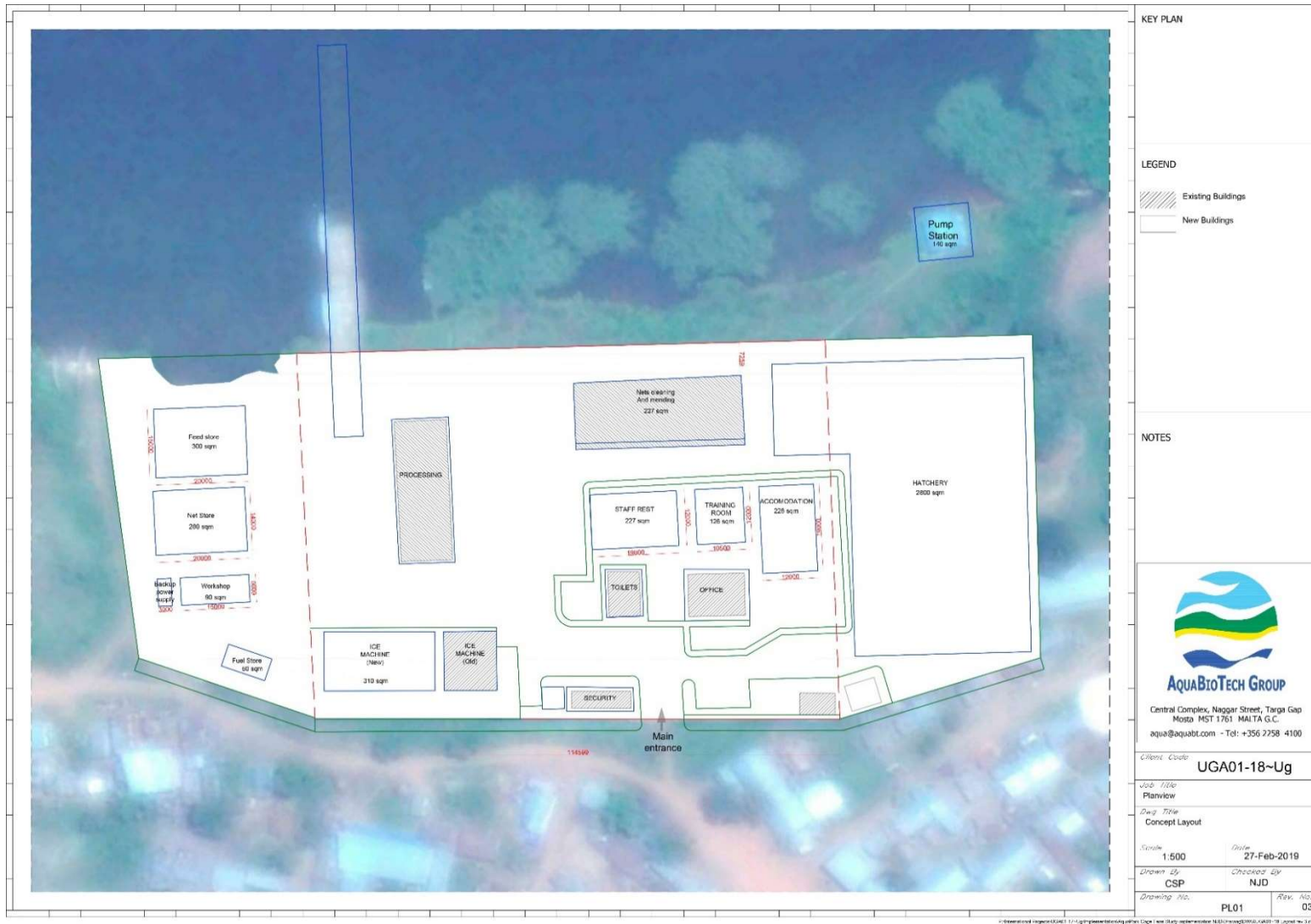
Figure 16: preliminary design layout of Mwena landing site presenting the current facilities and additional facilities required. This drawing is provided in A3 in annex 5.
