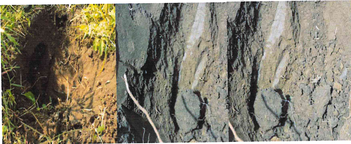
Figure 5; A hole used to test for water retention and the observed soil profile at Onekgwok
