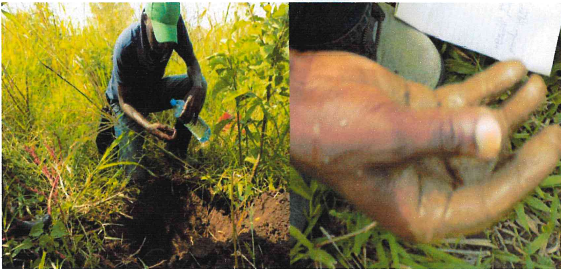
Figure 4; NaFIRRI Scientist testing soil texture and stickiness in the field at Onekgwok
