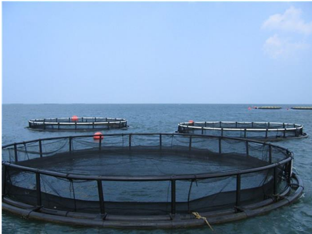
Figure 7; Circular HDPE cages which can be of diameter ranging between 10 to 20meter with a depth of 6 to 8m to used in Large Scale Holder operations
